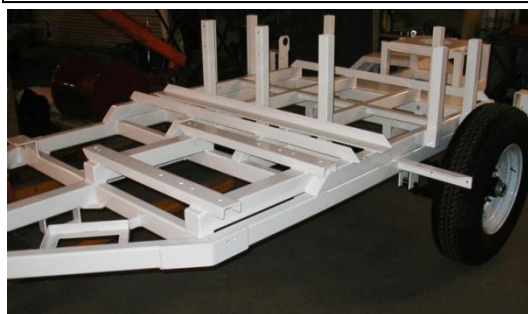
Below: U.S. crafted tubular steel frames are powder coated
