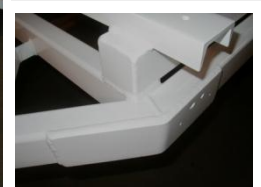
Gussets and "C" channels provide added stability
